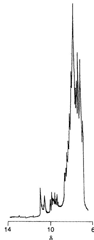
Fig. 3 Proton NMR spectrum of trans - [\text{MoBr}(\text{CHCHMe})(\text{dppe})_2] showing the partially resolved vinyl resonances, recorded at 25.0 °C in \text{CD}_2\text{Cl}_2
